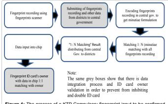
Figure 1: The process of e-KTP Compulsory fingerprint input to be confirmed from chip
