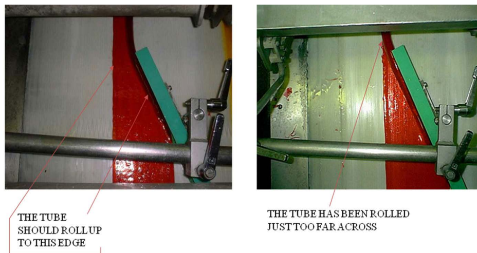
Figure 19.8. Incorrect plough set-up
