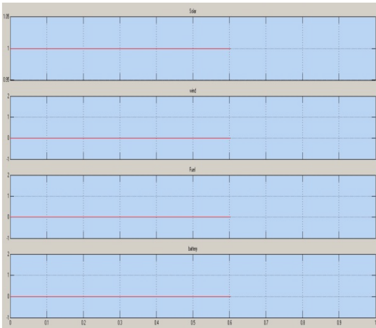
Figure 7: Solar ON state when load is below 1.2 A.
