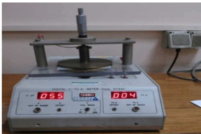
Figure 6: Capacitance tester (ASTM-D150), with two sputtered electrodes.
