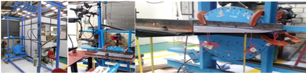
Figure 5: Mechanical test of the composite panel (a) in-house testing banc, (b) and (c) DIC setup.
