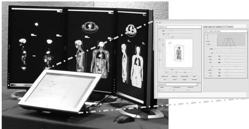
FIGURE 9.6 The touch screen is used to display the input interface that controls the display of data on the other three screens. In this example, the displays are used to visualize PET, fused PET/CT, and CT data, respectively (left to right). By separating the input controls, additional screen space is available to display the images.
