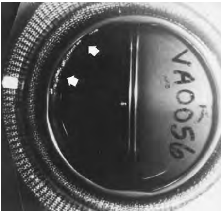
FIGURE 44.5 Cavitation bubbles visualized on the inflow side of the valves in vitro [Chandran et al., 1994a]: (a) Medtronic-Hall tilting disc valve; (b) Edwards-Duromedics bileaflet valve; (c) CarboMedics bileaflet valve.
