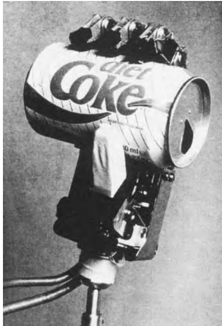
FIGURE 68.10 The Southampton hand prosthesis with four degrees of freedom in a power grip. An optical/acoustic sensor is mounted on the thumb. (Reprinted from Chappell, P.H. and Kyberd, P.J. 1991. J. Biomed. Eng. 13: 363, Figure 1.)
