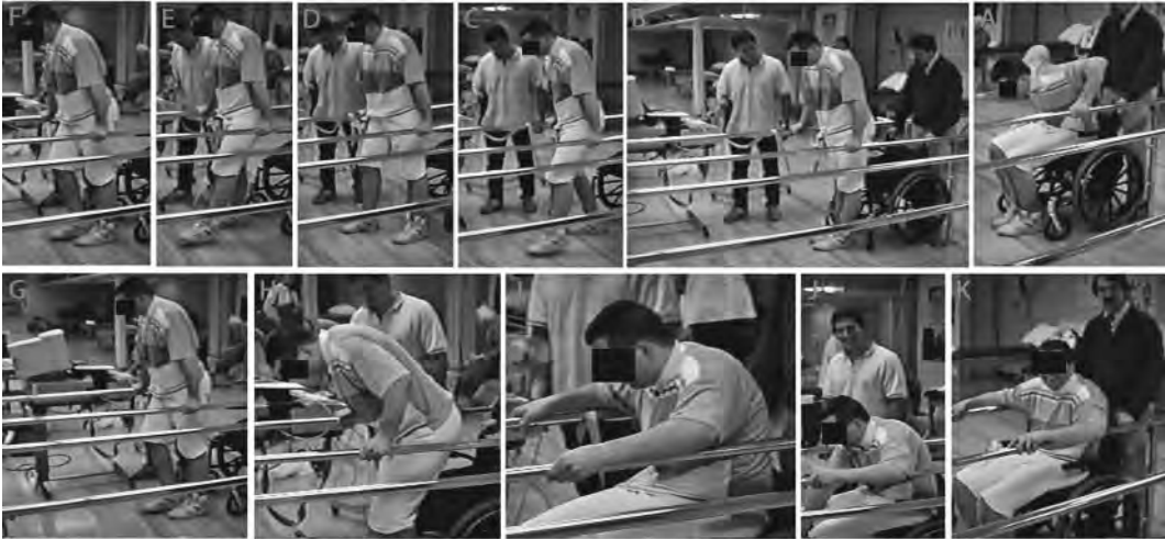
FIGURE 29.1 Series of still images from 4-channel FES gait sequence performed by author (DJJ) at MIT in 1990. (A) Subject bracing to stand, (B) Standing under FES control with computer controlled stimulator on the far left (L to R: author DJJ, subject, Allen Wiegner, PhD), (C) First step, (D) Second step, (E) Third step, (F) Fourth step, (G) Preparing to sit, (H) Sitting down, (I) Seated in wheelchair after walking, (J) Repositioning feet, (K) Smiling.
