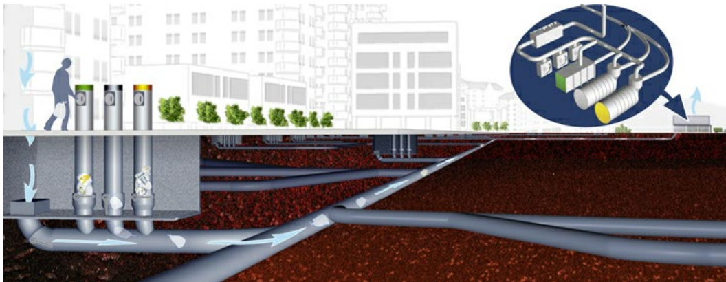
Figure 8.3 The AVAC system (Source http://www.envacgroup.com/ )
