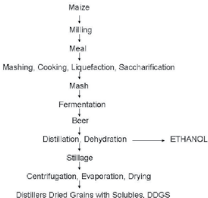
Fig 4.5 Ethanol production from maize (dry-grind process)
