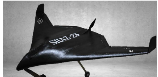
Figure 14: The final BWB prototype (5 ft wingspan).
