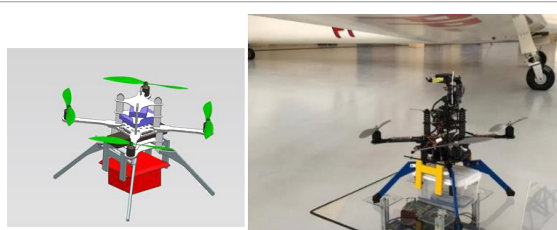
Figure 15: UAV's gripper attaching the box.
