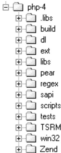
Figure 9.2 Main directory layout of the PHP source tree.
