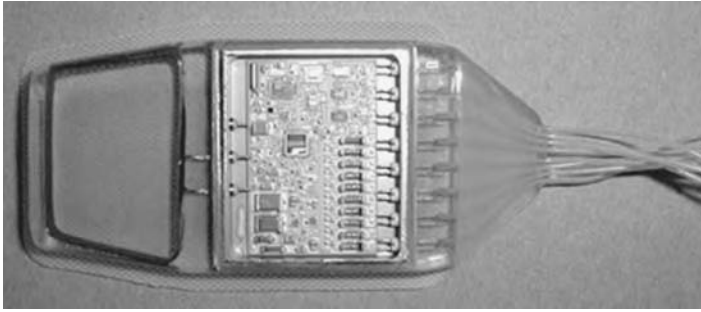
FIGURE 59.3 Photograph of a multichannel implantable stimulator telemeter. Hybrid circuit in titanium package is shown exposed. Receiving coil (left) is imbedded in epoxy resin together with titanium case. Double feedthroughs are seen penetrating titanium capsule wall on the right.
