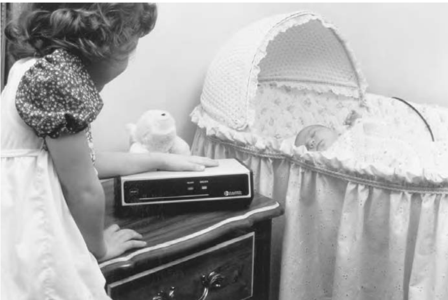
FIGURE 72.1 Infant apnea monitor used in a typical home setting. (Photo courtesy of EdenTec Corporation.)
