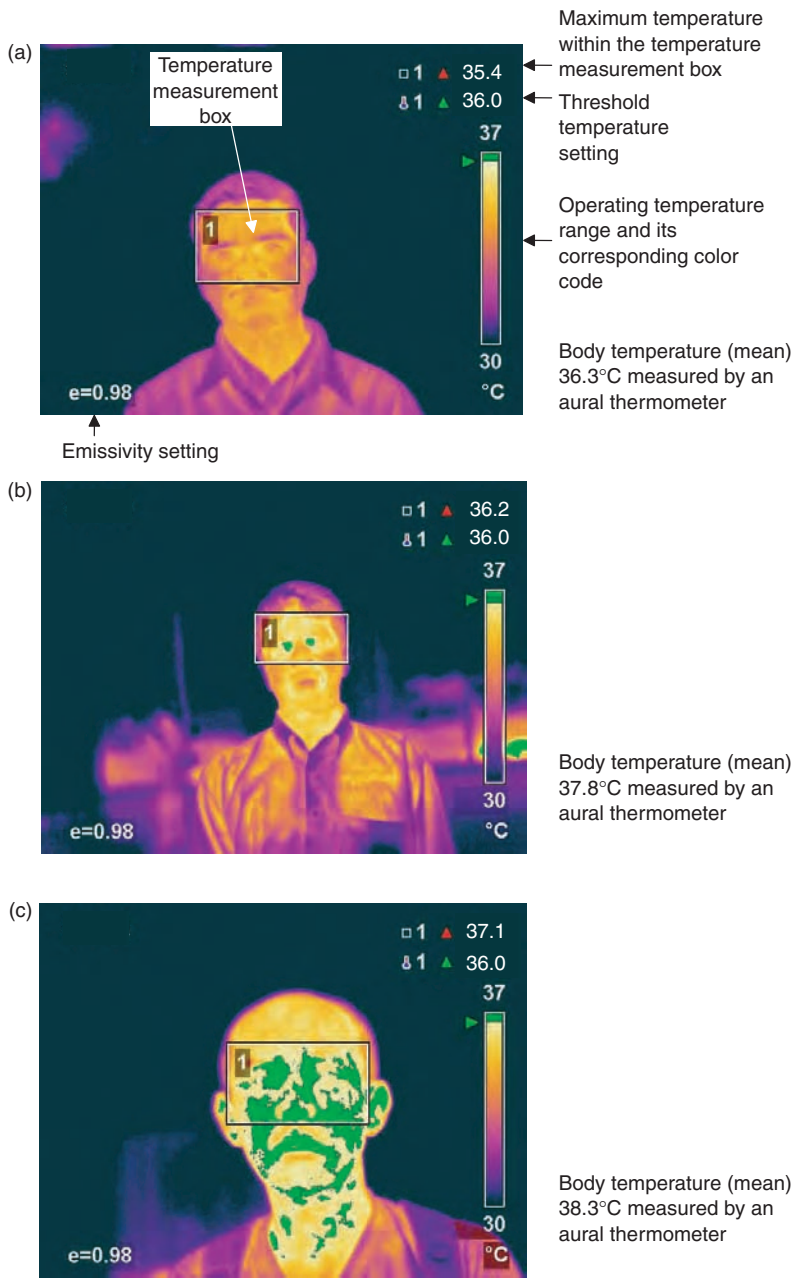
FIGURE 24.1 Examples of temperature profiles using thermal imager with temperature readings.
