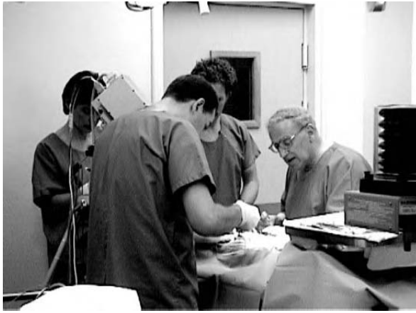
FIGURE 33.1 Typical set-up for a thermal imaging in surgery. The camera is tripod mounted toward the foot of the operating table and aimed at the surgical access site (camera visible over the left shoulder of the nearest surgeon).
