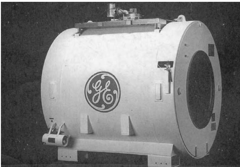
FIGURE 12.8 Superconducting magnet. This figure shows a 1.5-T whole-body superconducting magnet. The nominal warm bore diameter is 1 m. The patient to be imaged, as well as the RF and gradient coils, are located within this bore. (Courtesy of General Electric Medical Systems. Reprinted with permission from Schenck and Leue, 1991.)
