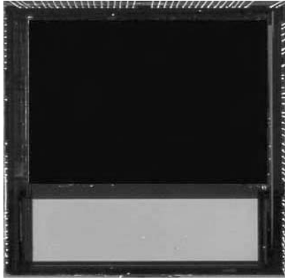
FIGURE 37.27 Focal planes with on-chip A/D converters have been demonstrated. This example shows a 900 \times 120 TDI scanning format array. Photo supplied by Lester Kozlowski of Rockwell Scientific, Camarillo, CA.
