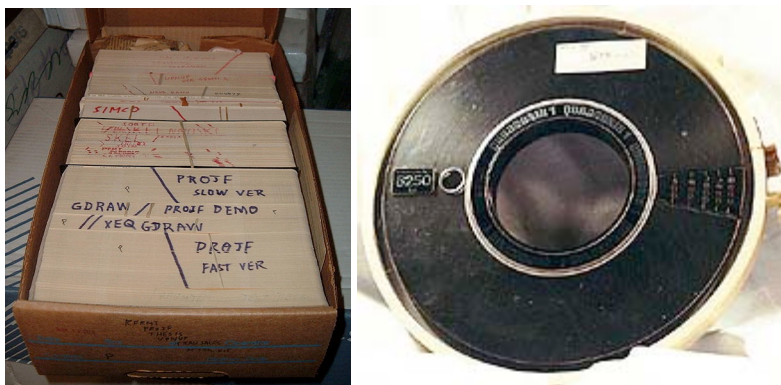
Figure 7. Old style databases: a box containing a set of punch cards (left) and magnetic tape (right). (Sources -- Left: Arnold Reinhold [ http://en.wikipedia.org/wiki/File:PunchCardDecks.agr.jpg ]; Right: Professor Gabriel Robins, University of Virginia [ http://www.cs.virginia.edu/brochure/images/mus_070.jpg ])
