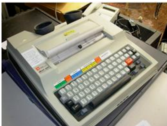
Figure 12. Texas Instruments Silent 700 terminal with acoustic coupler and thermal printer. (Source: http://www.flickr.com/photos/hckhckhck/124699193 )
