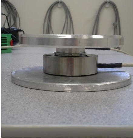
Figure 1. Lateral view of the force transducer enclosed within custom built metal plates.
