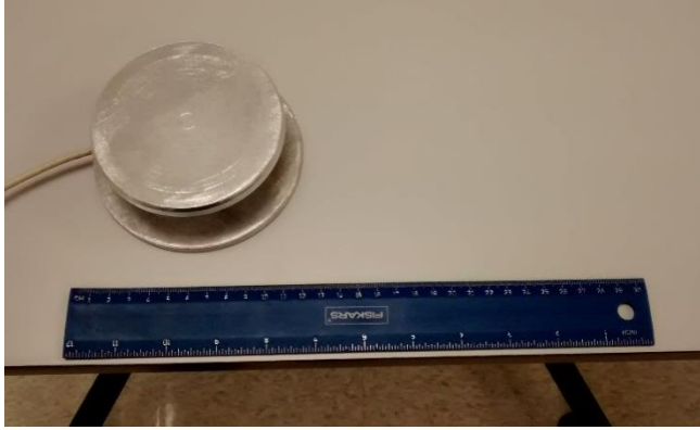
Figure A1. Aerial view of the force transducer encompassed in the metal casing, next to a 30 cm ruler.
