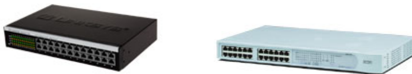
Fig 6b: 2 Examples of 24 port Switches
