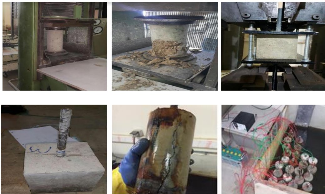
Fig.2: Compressive strength, pull out, and accelerated corrosion tests Reference: Photographed by the author November 2015
