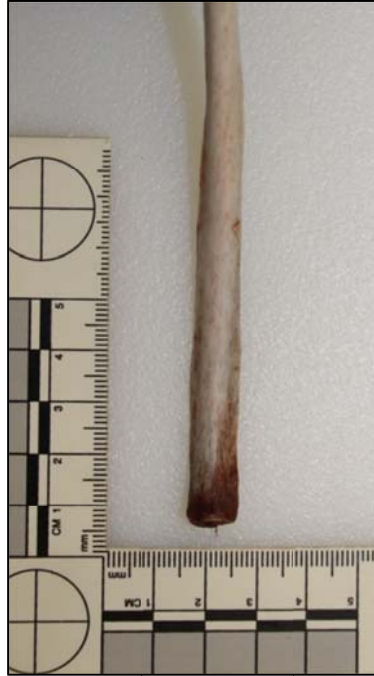
Figure D20: No rib fracture, medial aspect: Test 13-1L, 15-ply
