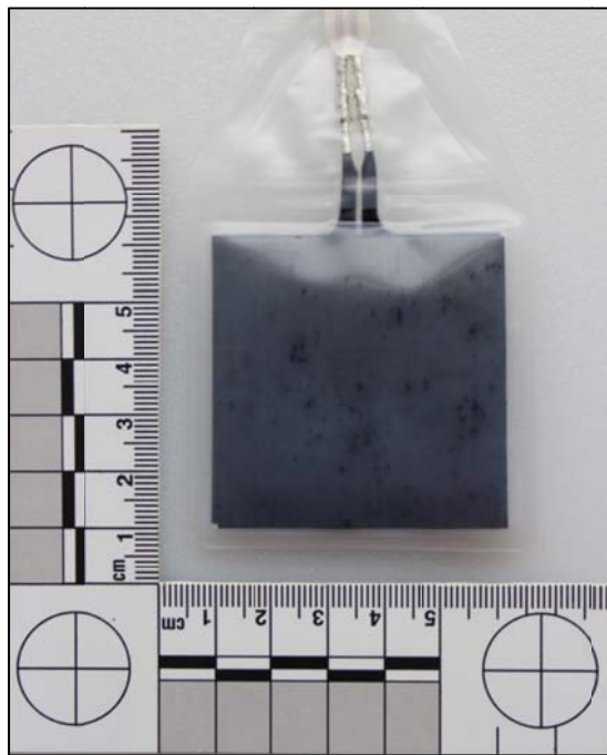
Figure 4.6: Polymer-on-polymer force sensor
