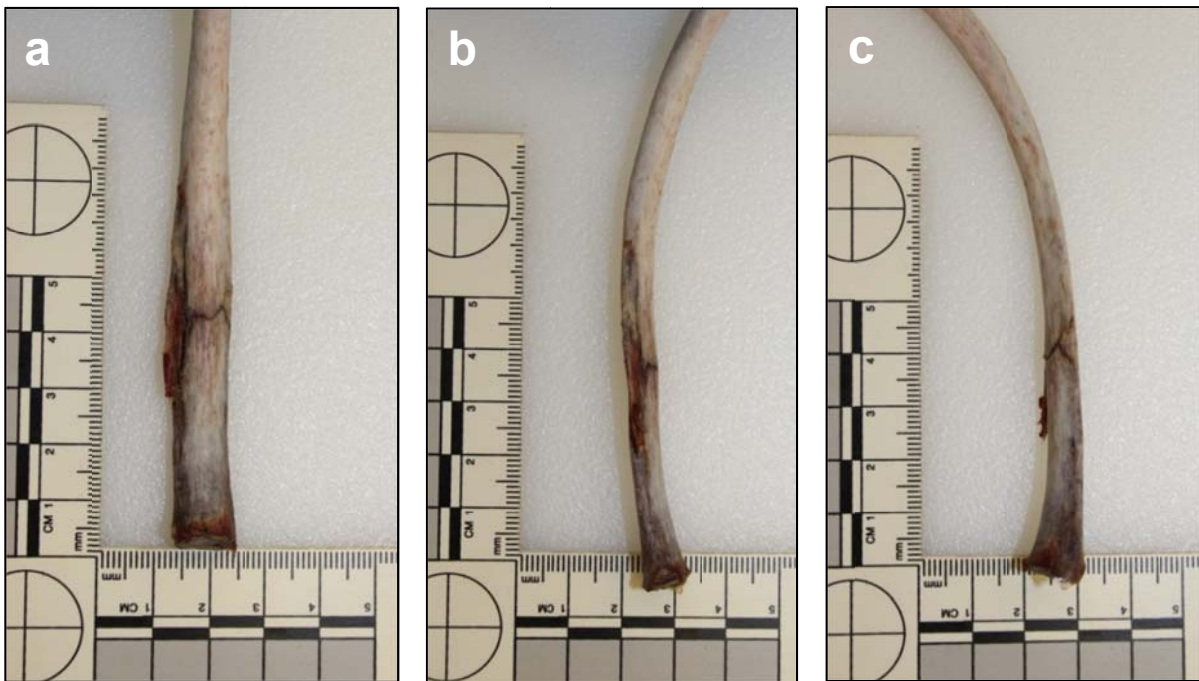
Figure D17: Rib fracture a) medial, b) cranial* and c) caudal* aspect (*incomplete butterfly fracture): Test 11-2R, 8-ply
