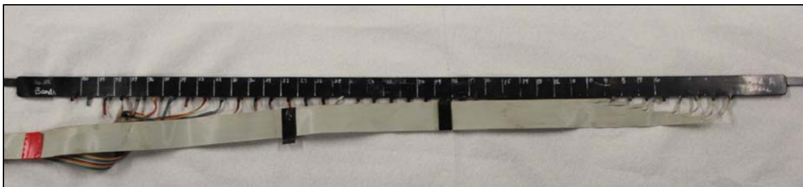
Figure 7.5: Forty-gage chestband schematic
