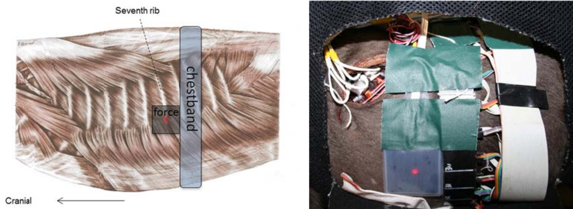
Figure 7.7: Positioning of chestband and force sensor with respect to impact site
