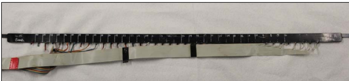
Figure 4.5: Forty-gage chestband schematic
