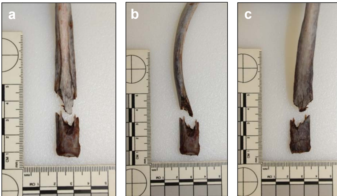
Figure D13: Rib fracture a) medial, b) cranial and c) lateral aspect: Test 9-2R, 8-ply
