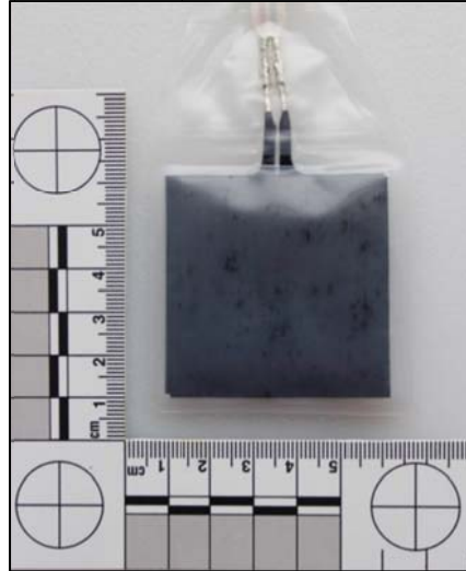
Figure 7.6: Polymer-on-polymer force sensor
