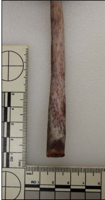
Figure D3: No rib fracture, medial aspect: Test 4-1L, 15-ply
