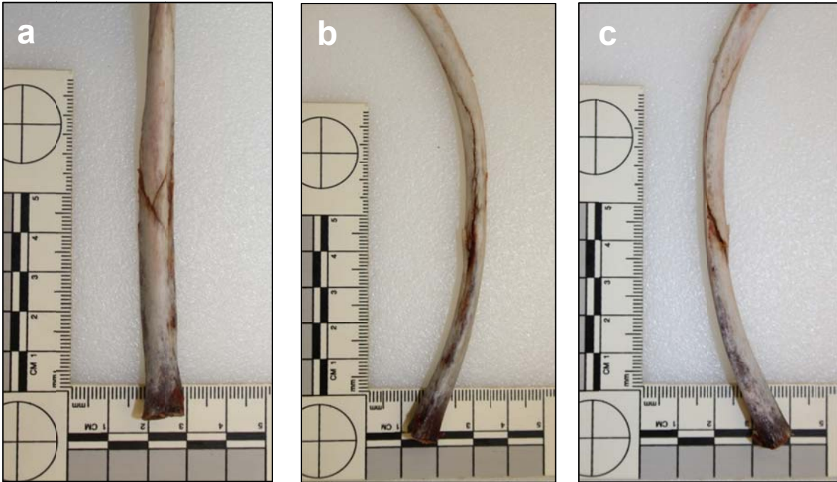
Figure D22: Rib fracture a) medial (incomplete butterfly fracture), b) cranial and c) caudal aspect: Test 14-1L, 15-ply
