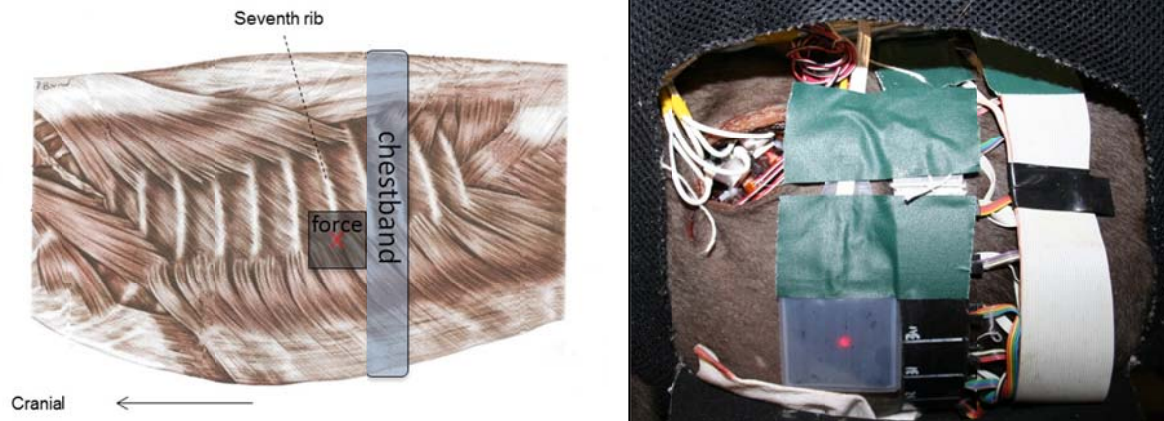
Figure 4.7: Positioning of chestband and force sensor with respect to impact site
