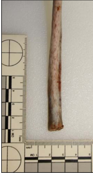
Figure D16: No rib fracture, medial aspect: Test 11-1L, 15-ply
