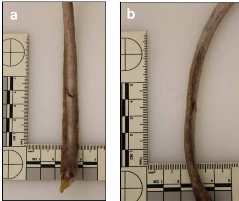
Figure D1: Rib fracture a) medial and b) cranial aspect: Test 2-2R, 8-ply
