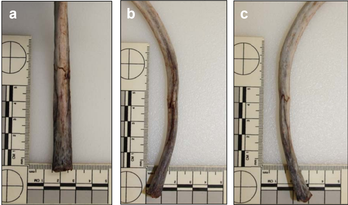
Figure D12: Rib fracture a) medial, b) cranial and c) caudal aspect: Test 9-1L, 15-ply
