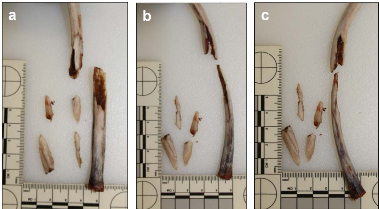
Figure D23: Rib fracture a) medial, b) caudal and c) cranial aspect: Test 14-2R, 8-ply
