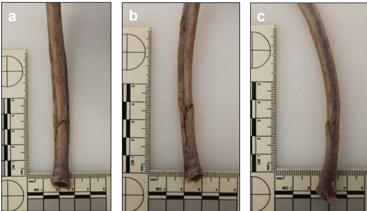
Figure D6: Rib fracture a) medial, b) cranial and c) caudal (incomplete butterfly fracture): Test 5-2R, 8-ply
