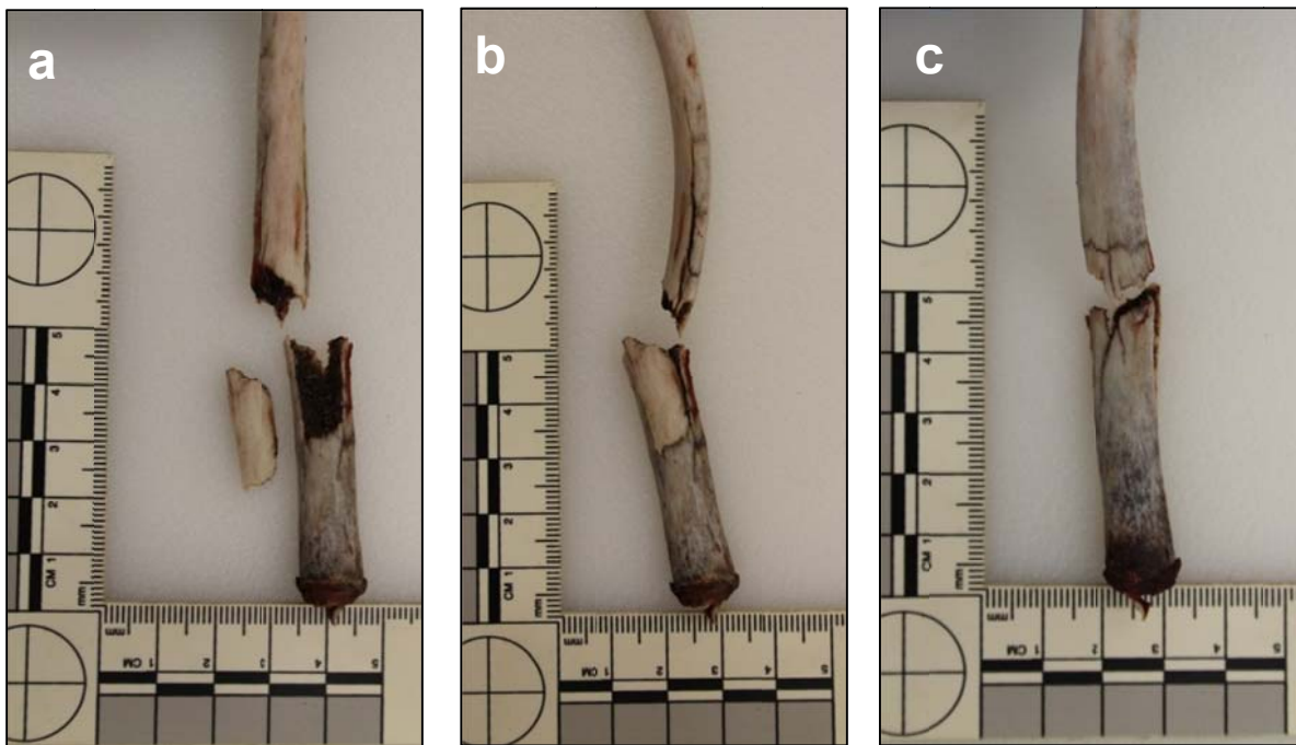
Figure D11: Rib fracture a) medial (butterfly fragment), b) caudal and c) lateral aspect: Test 8-2R, 8-ply
