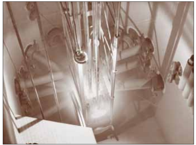
The FNR Nuclear Reactor core
