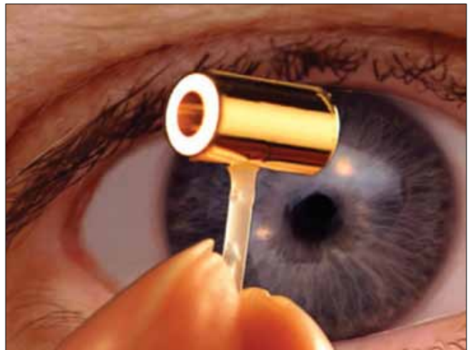
The target cavity containing the fusion pellet
