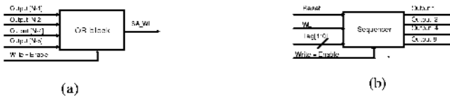
Fig. 2. (a) Block diagram of the OR block, (b) block diagram of the sequencer.
