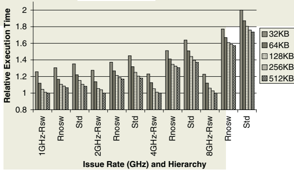
Fig. 2. Relative execution times (normalised: best at each issue rate = 1) as cache sizes vary with instruction issue rates.
