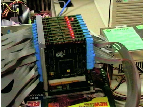
Fig. 1. An assembled Achilles router ‘stack’. Ten PCBs are installed in a bus backplane.
